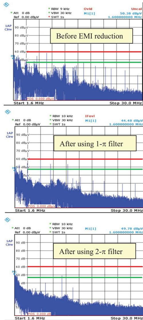
Figure 8: K4 EMI reduction by  $1-\pi$  &  $2-\pi$  filter (3 kV firing).
