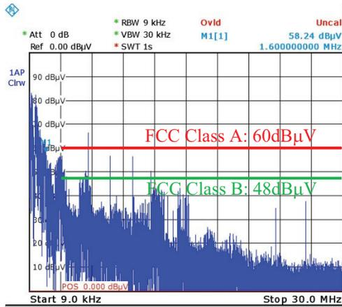
Figure 3: Kicker firing under 3 kV.
