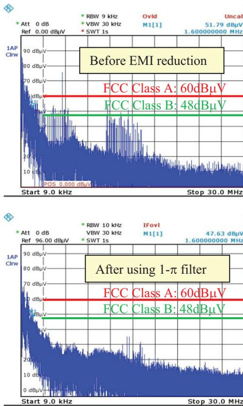
Figure 7: K2 EMI reduction by  $1-\pi$  filter (standby).
