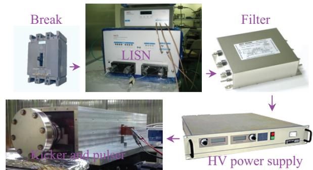
Figure 6: Experimental setup with EMI filter.
