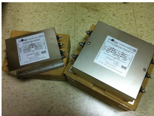
Figure 4: 3-Phase line filter (1- $\pi$  vs. 2- $\pi$ ).
