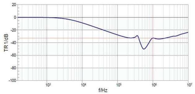
Figure 5a: Insertion loss of HUA-9010-2510 (1- $\pi$  filter).
