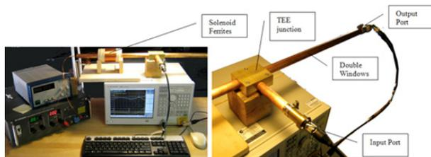
Figure 3: Experimental set-up used to evaluate ferrite materials.
