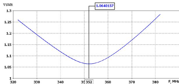
Figure 4: Shows the calculated VSWR at the RF input.
