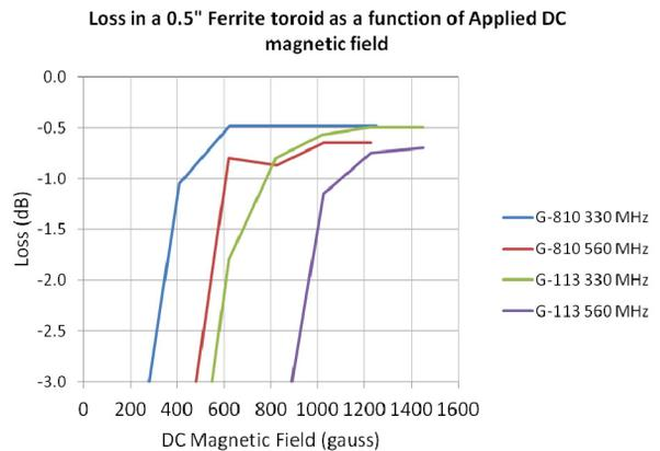
Figure 7: Shows the loss in a 0.5" thick ferrite toroid as a function of the applied DC magnetic field.
