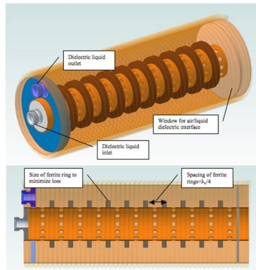
Figure 1: Schematic of the tuner section.
