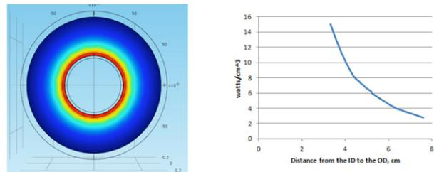
Figure 6: Loss profile for a ferrite toroid between the inner and outer conductor of EIA 3 1/8 coax.
