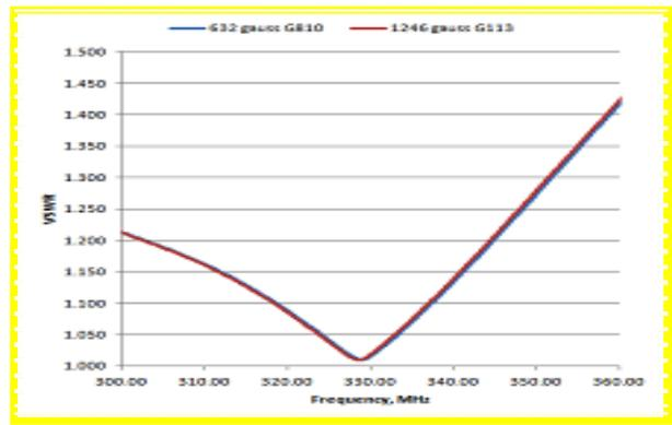
Figure 5: Shows the measured VSWR at the RF input.
