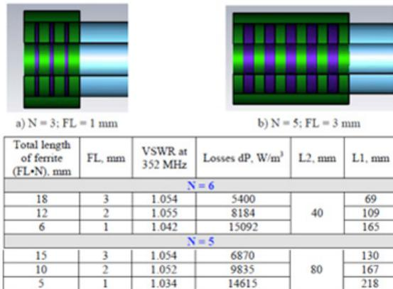
Figure 8: Sample loss calculations for the full power design of Phase II. L1 and L2 represent positioning information for the ferrites and the output window.
