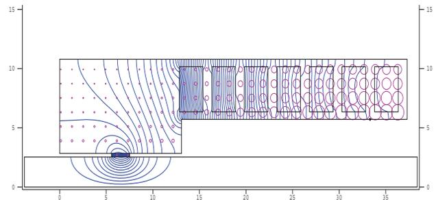
Figure 4: SUPERFISH simulation results with axis in units of cm. Resonance frequency of 30.296 MHz at  $\mu'_r = 53.4$ .
