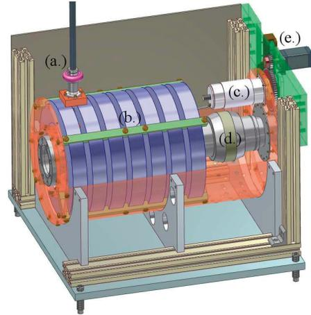
Figure 1: Cross-sectional drawing of the cavity design. (a.) rf drive point, (b.)  $M_4C_{21A}$  ferrite rings, (c.) vacuum capacitor, (d.) ceramic gap, (e.) capacitor tuning motor.
