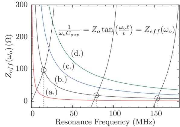
Figure 3: (a.) through (d.) corresponds to  $C_{\text{gap}}$  of 650 pF, 109 pF, 65 pF, and 25 pF, respectively. The solution with fundamental resonance frequency of 15 MHz exists when  $C_{\text{gap}} = 109$  pF.
