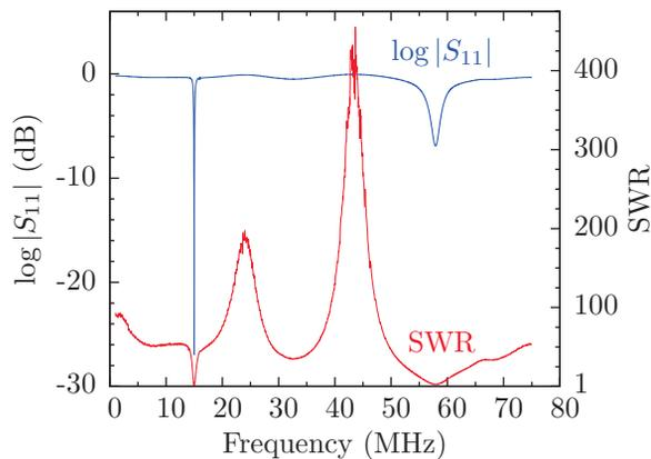
Figure 5: Cavity characterization with vector network analyzer where the SWR was measured to be 1.07 at 15 MHz.
