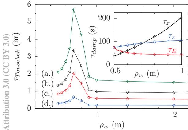
Figure 2: (a.) through (d.) are Touschek lifetimes varying with  $\rho_w$  and  $V_{\text{gap}}$  of 2 kV, 1 kV, 0.5 kV, and 0.1 kV, respectively. The subplot presents radiation damping times in the region of operational interest.
