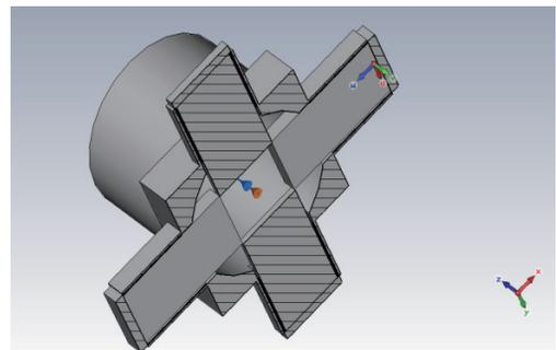
Figure5: CST model of CSNS primary collimator.
