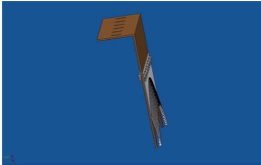
Figure7: Spring fingers for RF shield.
