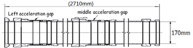
Figure1: Schematic diagram of RF cavity.
