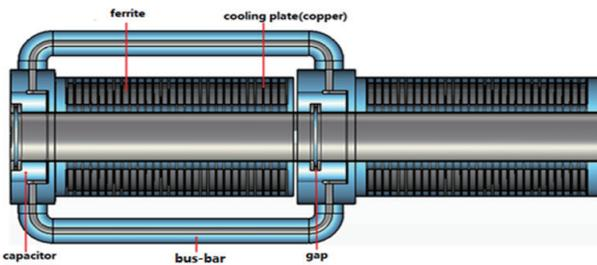
Figure 3: CST model of CSNS ring RF cavity.
