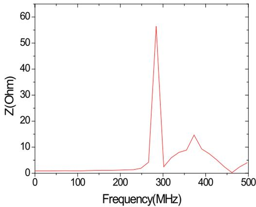
Figure 6: longitudinal impedance distribution of primary collimator with no RF shield.
