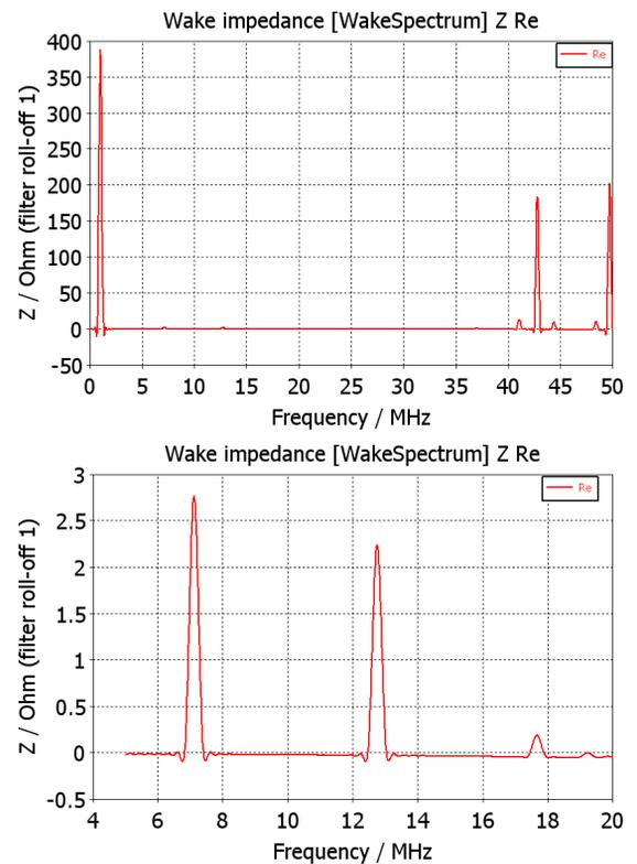
Figure 4: longitudinal impedance of RF cavity.
