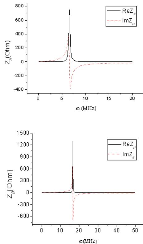
Figure 2: The longitudinal impedance of single gap for injection (up) and for extraction (down).
