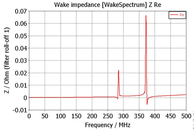
Figure 8: longitudinal impedance distribution of primary collimator with RF Shield.
