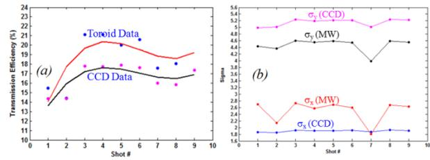
Figure 6: (a) Comparison of beam transmission efficiency calculated from CCD data and toroid, (b) comparison of beam between CCD data and multi-wire data during beam test done on summer 2012.
