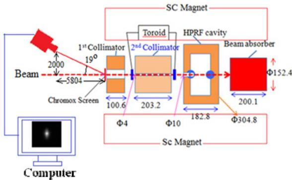
Figure 1: Schematic of HPRF cavity beam test at MTA.
