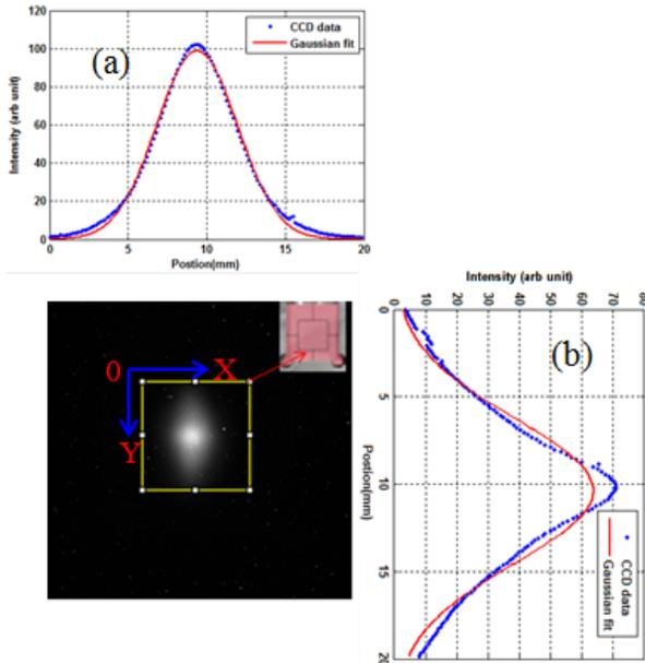
Figure 3: Beam image on Chromox-6 scintillation screen taken with CCD camera for 400 MeV proton beam. Horizontal (a) and vertical (b) beam profiles with Gaussian fit are also shown.
