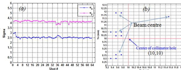
Figure 4: (a) horizontal beam width ( $\sigma_x$ ) and vertical beam width ( $\sigma_y$ ) at different beam shot number, (b) position of beam centre w.r.t centre of collimator hole at different beam shot.
