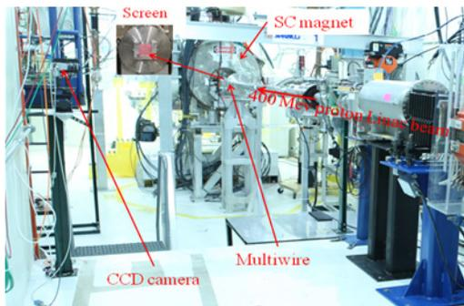
Figure 2: MTA beam line with Chromox-6 screen.
