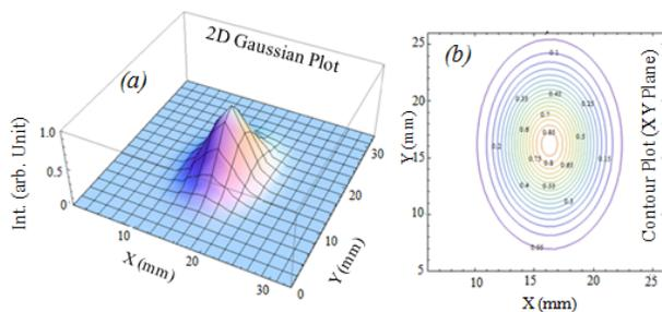
Figure 5: Two dimensional Gaussian distribution plot (left) of the beam image shown in Fig. 3 and its contour plot on X-Y plane (right).
