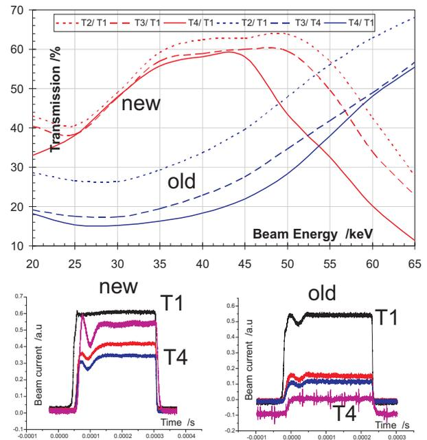
Figure 6: Transmission through the beamline, the current is measured with the 4 toroids. Input current at T1 is almost the same for both the new and old post acceleration. This implies less current density in the outer wings of the tail of the beam.
