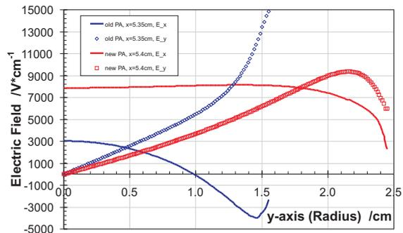
Figure 4: Radial field components of the two PA at the outlet of the protection electrode.  $E_x$  is the field component parallel to the beam axis and  $E_y$  is the radial (transversal) component.
