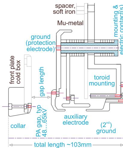
Figure 2: Cross section of the technical design of the new post acceleration. Mounted on 3 insulation pipes with spacers for alignment but here only one is shown.
