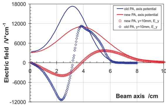
Figure 5: Beam axis potential of the two versions of the post acceleration shown for  $r = 0$  mm and  $r = 10$  mm. The latter is especially important to reduce aberration because most of the beam current density can be expected within  $\pm 8 \dots 12$  mm.
