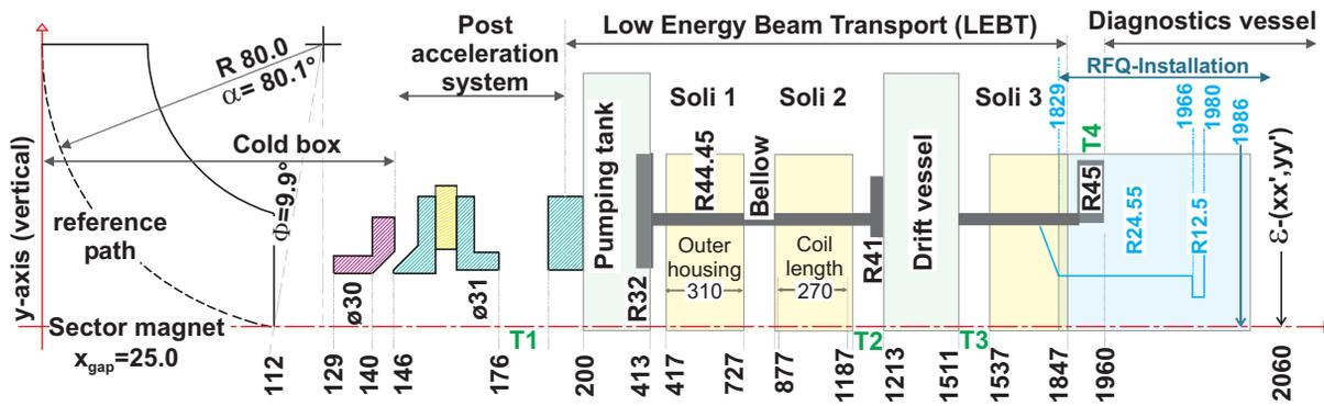
Figure 1: The beamline as it is at the moment for LEBT commissioning with a diagnostics vessel instead of the RFQ. Shown is the electrode design of the old PA.
