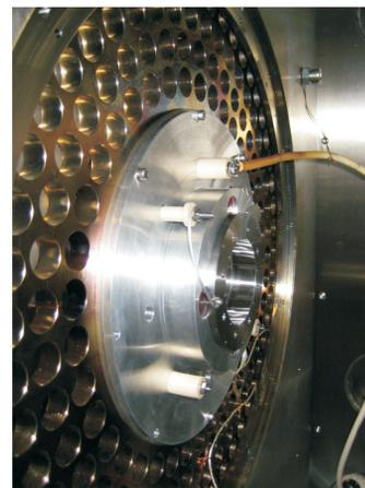
Figure 3: Top: The assembled PA with all 3 electrodes and connectors. Bottom: The PA mounted on the semi-permeable wall.
