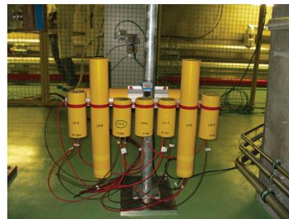
Figure 5: View of the detectors on the metallic cross in TSG45.
