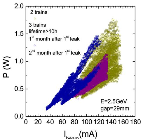
Figure 4: Variation over six years of the beam heat load reported as a function of the average beam current. Beam parameters:  $E = 2.5$  GeV,  $I_{beam} = 80 - 200$  mA. Undulator parameters: gap = 29 mm.
