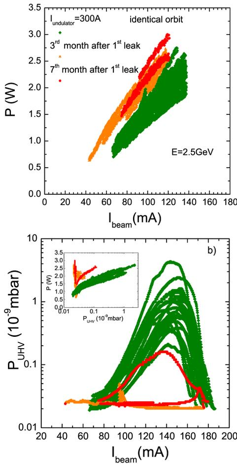
Figure 1: a) Variation over half a year of the beam heat load and b) of the UHV pressure reported as a function of the average beam current. In the inset of plot b), the beam heat load is shown as a function of the UHV pressure. Beam parameters:  $E = 2.5 \text{ GeV}$ ,  $I_{beam} = 80 - 200 \text{ mA}$ , three trains. Undulator parameters: gap = 8 mm, undulator current = 300 A.
