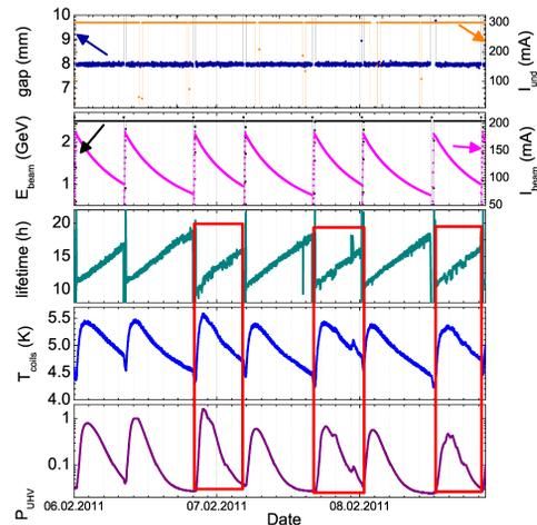
Figure 2: User operation run with 8 mm closed gap an 300 A current in the undulator. The undulator current and gap, the beam current and energy, the lifetime, the temperature of the coils and the UHV pressure are reported as a function of time.
