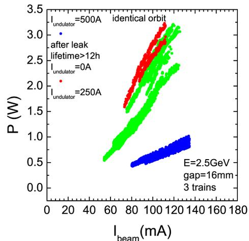
Figure 3: Variation over three years of the beam heat load reported as a function of the average beam current. Beam parameters:  $E = 2.5 \text{ GeV}$ ,  $I_{beam} = 80 - 200 \text{ mA}$ , three trains. Undulator parameters: gap = 16 mm, undulator current = 0 – 500 A.
