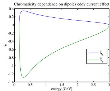
Figure 7: Chromaticities induced by eddy currents on the dipoles vacuum chambers due to the ramping process.
