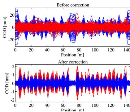
Figure 5: Closed orbit distortion for one hundred machines with random errors. Red lines represent the vertical and blue lines, the horizontal plane.
