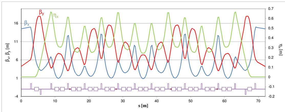
Figure 2: Optical functions of one super-period of the Booster.
