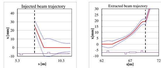
Figure 4: Injected and extracted beam trajectories. In red, the beam center and in blue  $\pm 3$ -beam size at injection/extraction. The point where beam center crosses the axis indicate the positions of the kicker and the vertical line the end/beginning of the thin septa.
