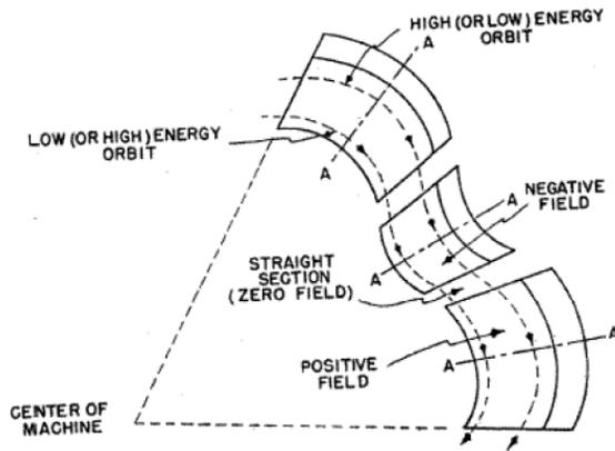
Figure 1: Schematic figure of a radial-sector FFAG [6]. As the beam is accelerated, the orbit moves to outside.
