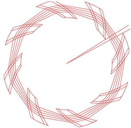
Figure 2: Spiral-sector FFAG and its orbits [7]. Again, the beam orbit moves outside, as it is accelerated.
