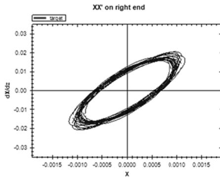
Figure 3: Optimized emittances in the plane  $(x, x')$ .
