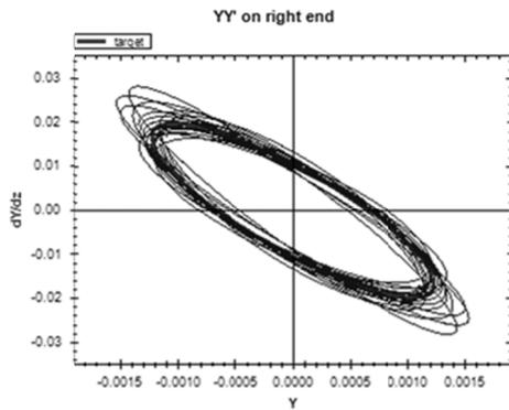
Figure 2: Initial emittances in the plane  $(y, y')$ .
