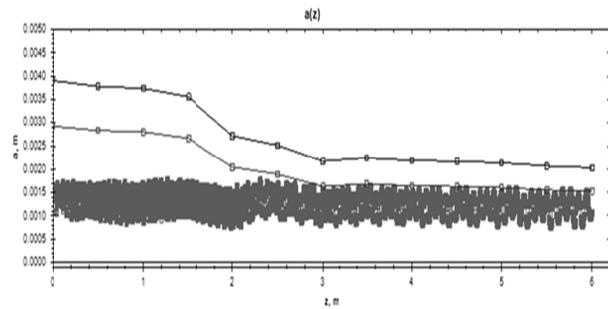
Figure 6: Optimized radius of the channel and beam envelopes.
