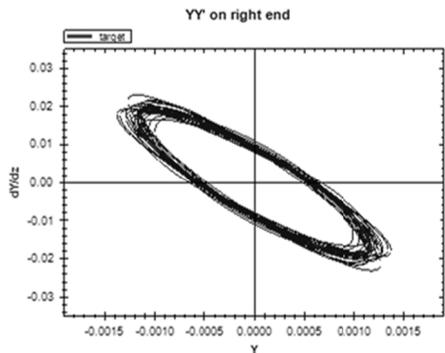
Figure 4: Optimized emittances in the plane  $(y, y')$ .
