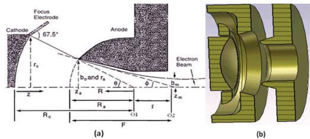
Figure 1: a) Spherical diodes analytic geometry [4] b) High-perveance gun geometry.
