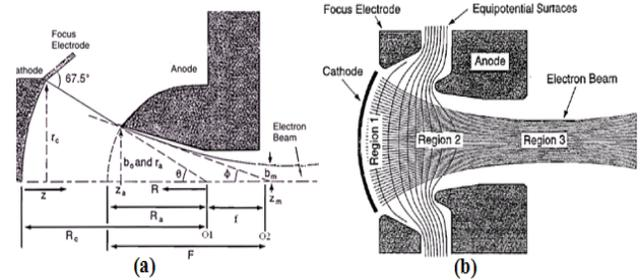
Figure 4: a) Pierce design geometry. b) Trajectory and different regions in this design [2].
