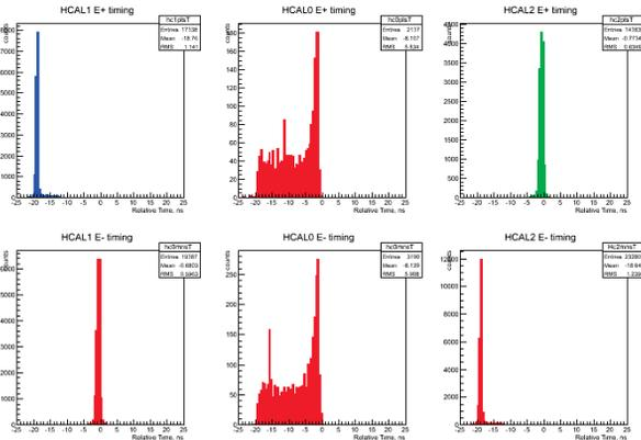
Figure 7: Difference in flight time of B-H muons when compared with a track arriving from the IP in time with the beam crossing. The top (bottom) row show time differences from  $\mu^+$  ( $\mu^-$ ) beams. The columns correspond to the backward, central and forward calorimeters.
