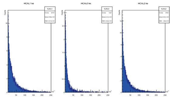
Figure 5: Kinetic Energy distribution of B-H muons entering the backward (left), central (center) and forward (right) hadron calorimeters. The KE is in GeV.
