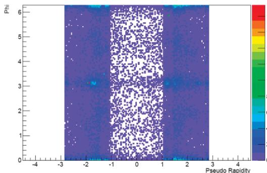
Figure 3: Muon hits in the calorimeter as a function of the detector physics variables:  $\phi$  and  $\eta$ .
