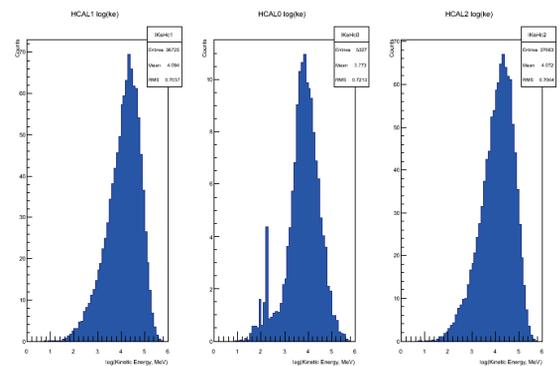
Figure 6:  $\log_{10}(\text{KE})$  distribution for B-H muons entering the backward (left), central (center) and forward (right) hadron calorimeters. The KE is in MeV.
