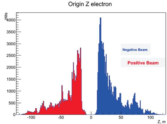
Figure 4: Origin of the muons that reach the detector calorimeter.
