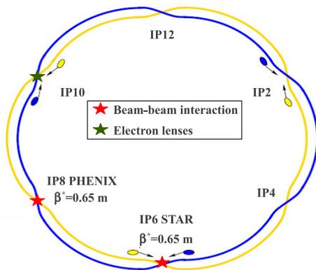
Figure 1: Layout of the RHIC collider. The colliding IPs are denoted by the red stars, the head-on compensation by the green star.
