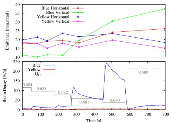
Figure 4: Tune scan towards the 2/3 resonance with colliding beams.
