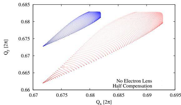
Figure 2: Tune footprint computed with BeamBeam3D for an intensity of  $3.0 \cdot 10^{11}$  protons per bunch with and without compensation.
