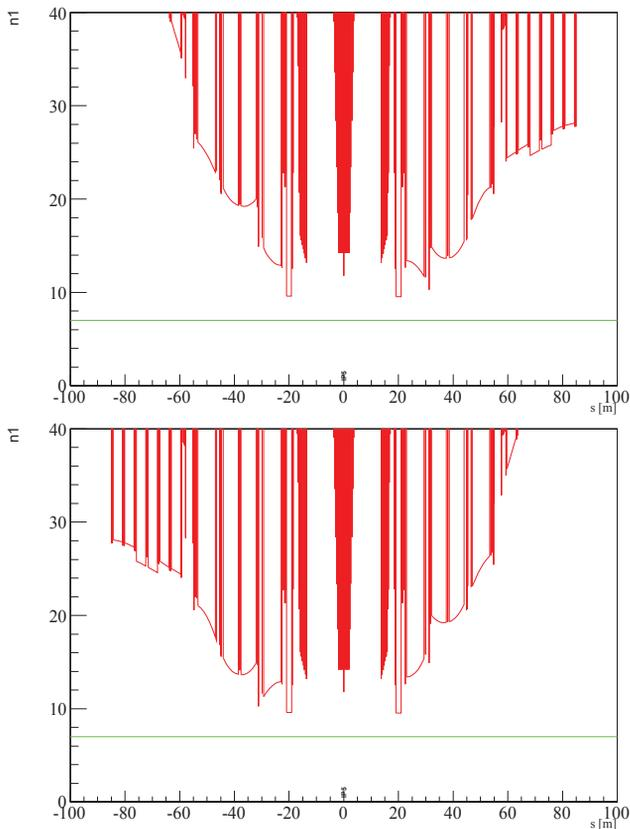
Figure 3: Aperture at 4 TeV, for the design emittance  $\epsilon_N = 3.75 \mu\text{m}$  at  $\beta^* = 500 \text{ m}$  around IP5 including  $\pm 2 \text{ mm}$  parallel separation. Top is for beam 1 and bottom for beam 2.
