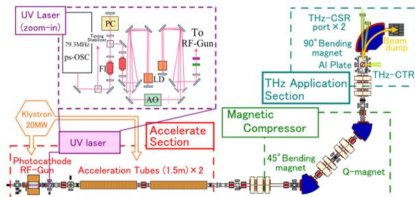
Figure 3: S-band linac beam line at AIST, Japan.
