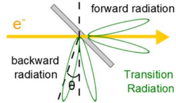
Figure 5: Scheme of transition radiation.
