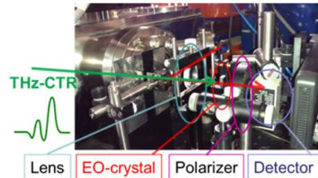
Figure 10: Experimental setup of the THz-CTR-TDS system with EO sampling method.
