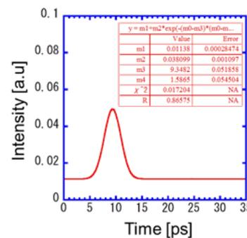
Figure 11: Measured THz temporal waveform (Gaussian fitted).
