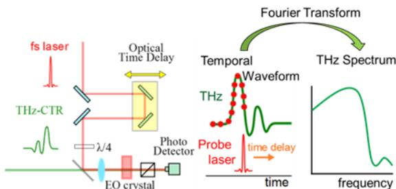
Figure 9: Schematic diagram of THz-CTR-TDS system with EO sampling method.
