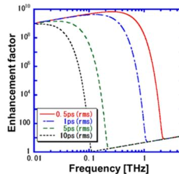
Figure 2: Enhancement factor of CSR as a function of its frequency by changing the bunch length.
