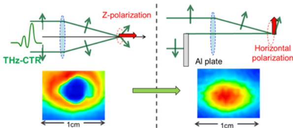
Figure 8: Polarization control of THz-CTR.
