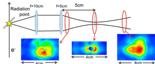
Figure 7: Profile changes of the THz-CTR electric field.
