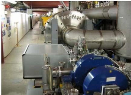
> Normal conducting 1.3 GHz RF gun
