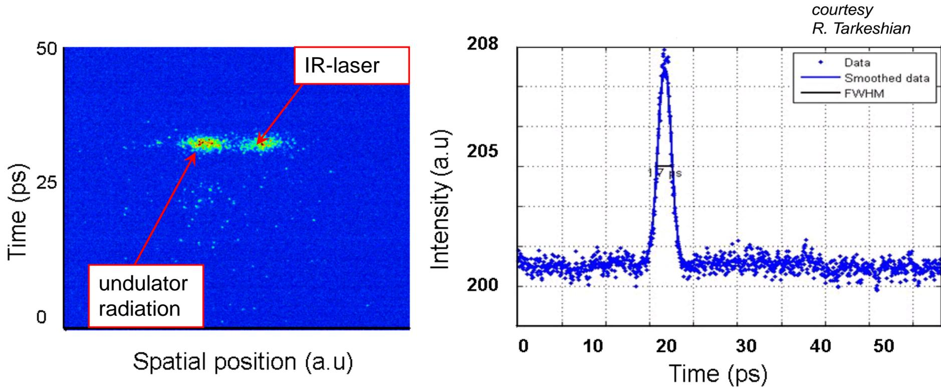
Temporal overlap ( $\sim 0.5$  ps) between the **HHG drive laser pulse** and **spontaneous undulator radiation** measured with the streak camera
