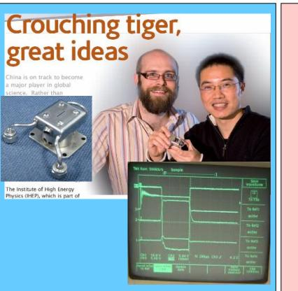
H- ion source: four H- ion source bodies were fabricated at IHEP and test at ISIS with a satisfactory results (55mA pulse current ).
