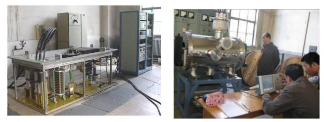
The pulse power supply uses Blumlein type pulse forming network to get a short pulse with a current of 5840A and a flattop of better than  $\pm$ 1.5%
