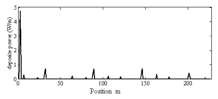
In case of no beam collimation, the total beam loss is small, but the maximum local beam loss is over 5W/m.
