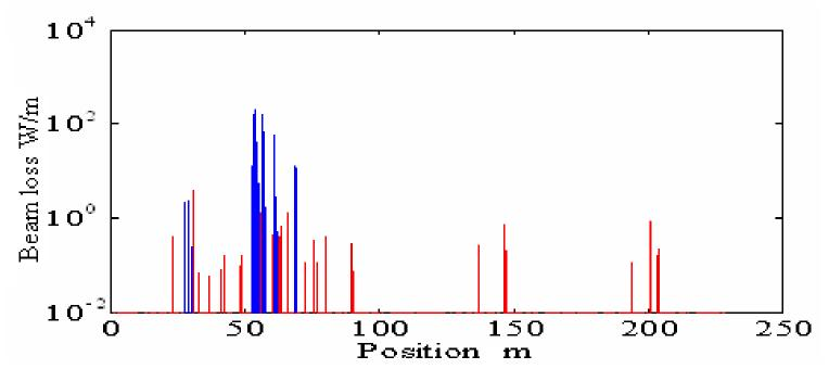
Beam loss distribution in the RCS with transverse and momentum beam collimation, total beam loss is about 5%, and the collimation efficiency is more than 96%
