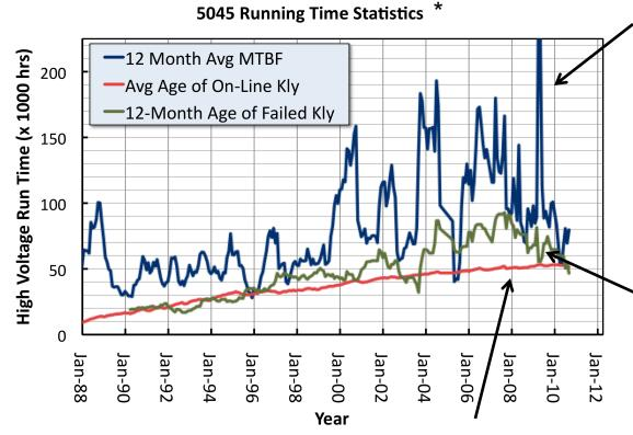
Average Age of On-Line Klystrons: total accumulated HV hours to date of the 245 currently installed 5045 klystrons divided by 245- 52,000 hrs **12 Month Avg MTBF**: total HV hours accumulated on all klystrons during the previous 12 months divided by the total number of failed klystrons during the same period – **80-90,000 hr**
