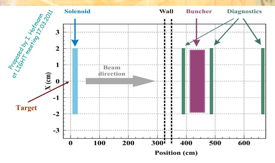
On the base of presented beam dynamics simulations the buncher will be shifted closer to the solenoid.
