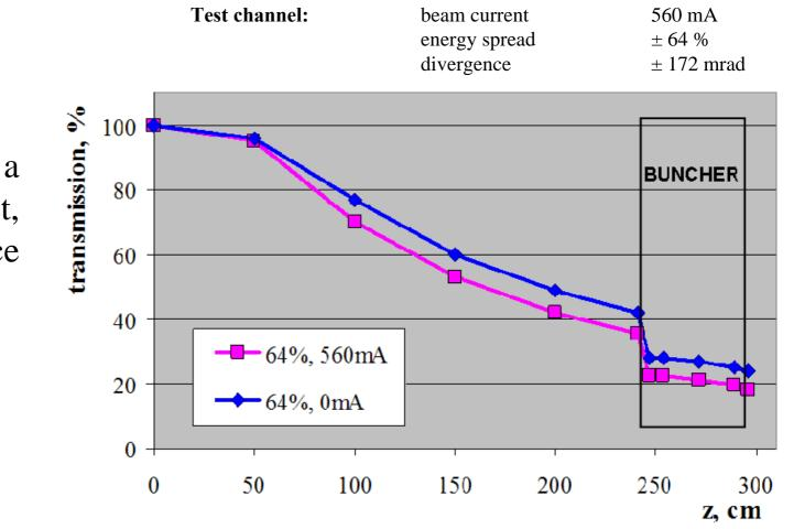
Behind a small area of a few mm from the target, an influence of the space charge is relatively low.
