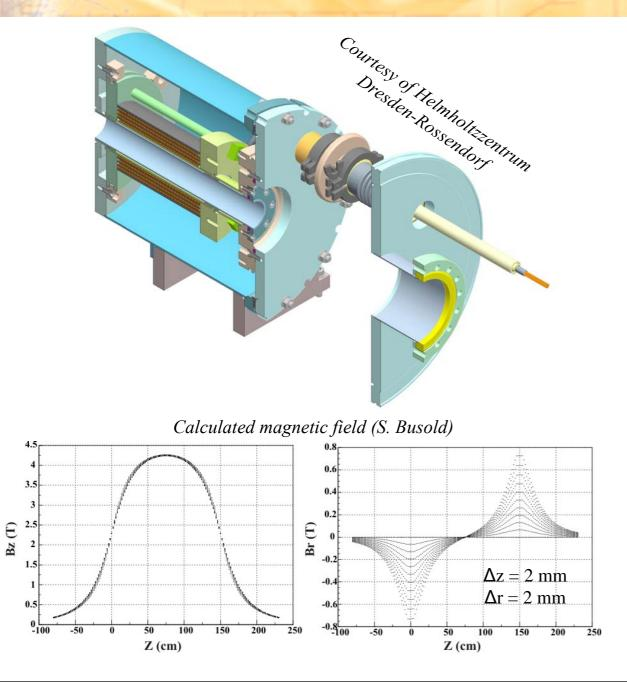
Use of the measured at GSI 3D magnetic field is foreseen for the further study
