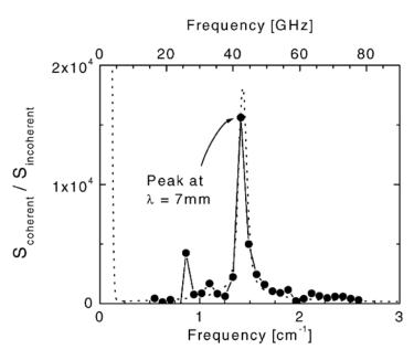
Fig. 4. (Symbols and solid line): measured spectral content of the coherent emission, relative to the incoherent synchrotron spectrum (ratio of spectra shown in Fig. 3). The small peak near  $0.8\,\mathrm{cm}^{-1}$  is probably due to poor S/N for the incoherent spectrum. Dotted line: modeled spectral content, including a non-observable Gaussian component, centered at zero frequency, for the overall bunch shape.
