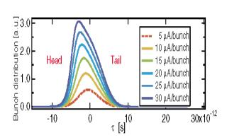
FIG. 1 (color online). Calculated equilibrium longitudinal distribution for different currents per bunch using the shielded SR wake. BESSY II case with a natural bunch length of 2.5 ps.
