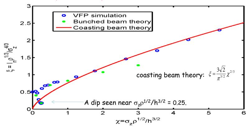
Threshold  $\xi^{th}$  becomes a function of the shielding parameter  $\chi = \sigma_z \rho^{1/2}/h^{3/2}$ . Simulation was carried out by K.Bane, Y.Cai, and G. Stupakov, PRSTAB 13, 104402 (2010). For a long bunch, the coasting beam theory agrees well with the VFP simulation.
