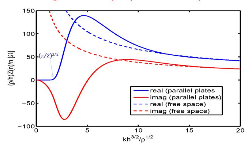
The scale defines the strength of impedance and the location of the peak defines where the shielding effects start.
