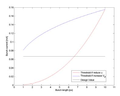
An illustration using PEP-X nominal parameters:  $f_{rf}$  = 476 MHz,  $V_{rf}$ =8.3 MV,  $f_{rev}$  = 136.312 kHz,  $\sigma_z$ =3 mm,  $I_b$ =0.067 mA.
