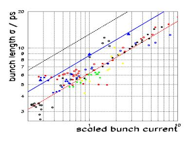
Figure 2: Scaled bursting threshold current  $\tilde{I}$  and bunch length  $\sigma_0$ . Blue line: theory; blue triangles: BESSY II data; circles: MLS data. All data are measured with a liquid He cooled InSb detector of one MHz frequency response.
