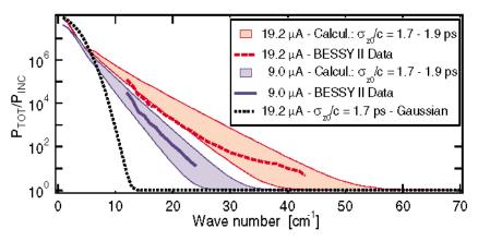
FIG. 2 (color online). CSR gain as a function of the wave number  $1/\lambda$ . The BESSY II data for two different currents per bunch are compared with the shielded SR calculation and with the curve for a Gaussian distribution of the same length.
