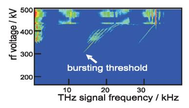
Figure 1: MLS THz signals at the bursting threshold. Vertical axis: applied rf-voltage amplitude, horizontal axis: frequency of the detected THz signals. The colour indicates the THz signal intensity.
