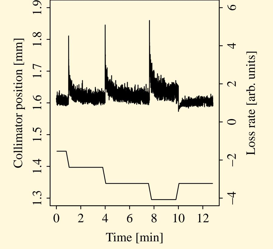
**Figure 2:** Example of the response of local loss rates to inward and outward collimator steps.
