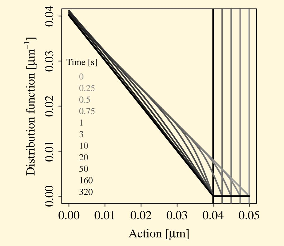
are summarized in Table 1. Every 2 to 3 minutes, the F48 vertical antiproton collimator was moved inward by 50  $\mu$ m in 0.2 s. At the location of the collimator the amplitude function was  $\beta_y = 29$  m and the r.m.s. beam size was  $\sigma_y = 320 \ \mu$ m.
