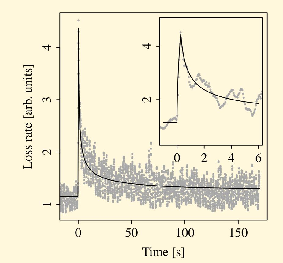
**Figure 5:** Measurements of the transverse beam diffusion rate with a vertical antiproton collimator scan (Tevatron Store 8527, 25 February 2011).
