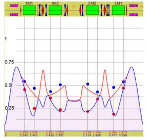
Figure 6: Beam sizes (mm) around the lattice.
