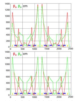
Figure 5: Lattice functions obtained by ORM analysis before and after lattice correction.
