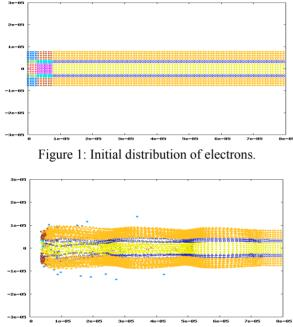
Figure 2: Distribution of electrons after 2,000 time steps.
