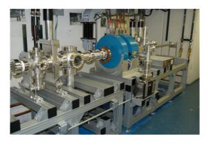
Figure 1: The new AWA RF gun (between the blue solenoids) commissioned, initially with a copper photocathode, which was later replaced with a Cesium Telluride photocathode.
