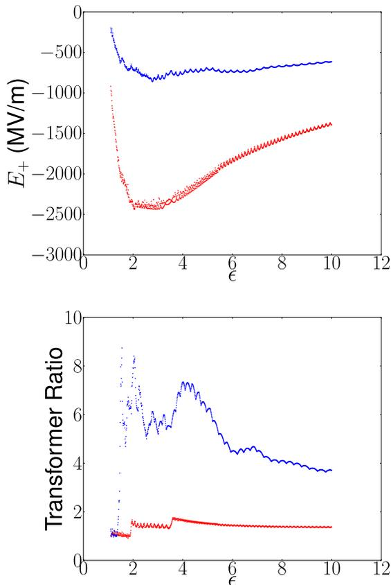
Figure 4: Accelerating field  $E_+$  (top) and transformer ratio  $\mathcal{R}$  (bottom) as a function of  $\epsilon$ . The blue and red traces respectively correspond to the current profile shown in Fig. 2 and 3. For these calculations,  $(a, \delta) = (20, 60) \mu\text{m}$ .
