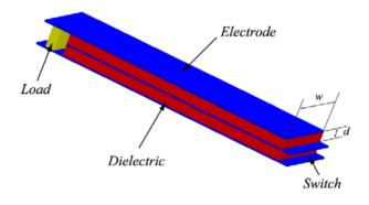
Figure 1: Compact parallel-plate Blumlein pulse-forming line configuration.
