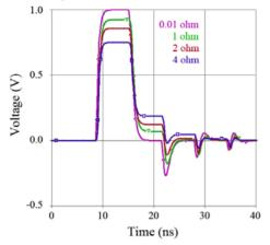
Figure 3: Output waveform from a single Blumlein for various switch on-resistance.
