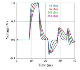
Figure 4: Output waveforms for various Blumlein impedance on a matched resistance connected in parallel with a 15 pF capacitance.
