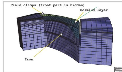
Figure 4: TOSCA model of multi-layer superferric magnet. (clamp in front and coils are hidden)
