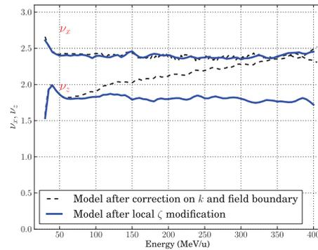
Figure 5: Minimization of tune shift in the ring during optimization procedures.
