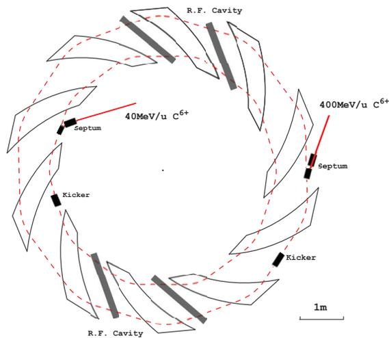
Figure 3: Schematic plan of the spiral FFAG ring for carbon therapy
