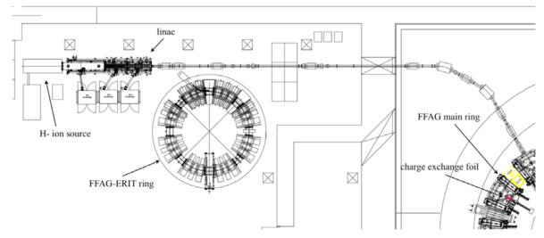
Figure 1: Schematic layout of beam transport line from H<sup>-</sup> linac to FFAG main ring.
