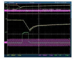
Figure 7: Signal of multi-turn injected beam. Yellow line is circulating beam signal, green line is chopper signal and pink line is signal of output rf voltage. From Fig. 7, circulating beam current was increase during multi-turn injection. However slow beam loss is observed. The reason for such beam loss, the longitudinal mismatch between the injection long pulse beam and rf bucket.
