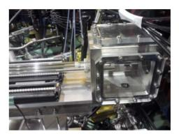
Figure 5: Photograph of installed foil installer machine with mounted carbon stripping foil. The thickness of this foil is  $20 \ \mu$  g.cm<sup>-2</sup>.
