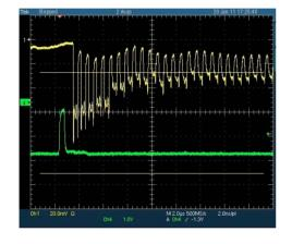
Figure 6: Beam signal of bunch monitor (yellow). Green signal is chopper output signal.
