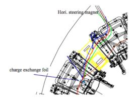
Figure 4: This figure is a H<sup>-</sup> injection orbit within main ring(red line). Brown line is a closed orbit of circulating beam.
