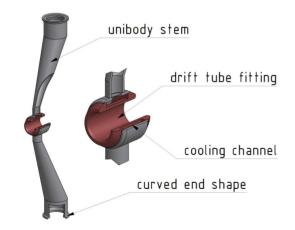
Figure 3: Cross sectional view of an inclined stem with a detail of the drift tube
