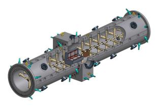
Figure 1: 3D-View of the coupled prototype cavity
