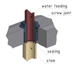
Figure 4: Cross sectional view of deatiled stem tank connection
