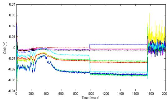
Figure 5: Closed orbit measurements along one cycle in the different horizontal pickups.
