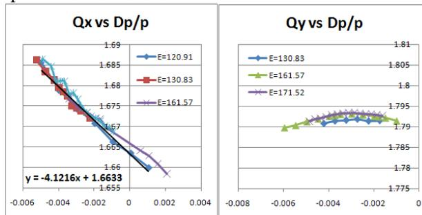
Figure 4: Horizontal (left) and Vertical (right) chromaticity measurements for some proton energies.
