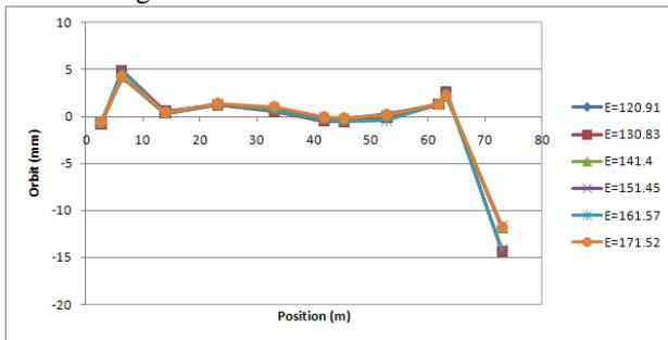
Figure 8: Horizontal closed orbit with the 5 magnets bump, for 6 beam energies between 120MeV to 170MeV.
