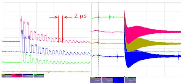
Figure 1 - Multiturn injection measured on three pick-ups without adiabatic trapping with 1 $\mu\text{s}$  beam and 30 $\mu\text{s}$  beam.
