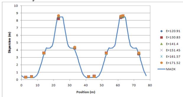
Figure 3: Horizontal dispersion measurements made at several energies compared with the theoretical value computed with MADX.
