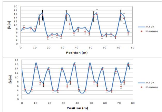
Figure 9: Measured and simulated (MADX)  $\beta_x$  and  $\beta_y$ .
