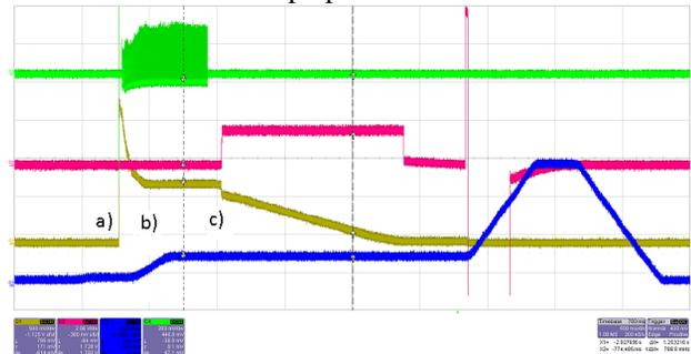
Figure 2: Signals shown on the control room scope: DCCT, B field, Pickup, Betatron core voltage. The main machine cycle phases are identified: a) injection, b) acceleration ramp, c) start extraction.
