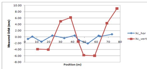
Figure 6: Closed orbit in the ring without steerers. In the horizontal plane the dispersive contribution is subtracted.
