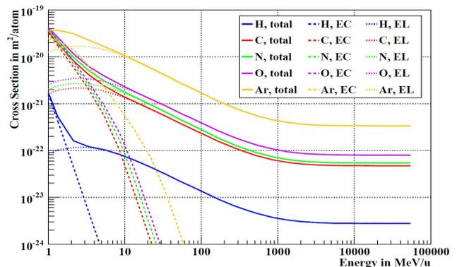
Figure 2: Calculated cross sections for ionization and electron capture of U<sup>28+</sup>-ions as a function of beam energy for various target (residual gas) atoms.
