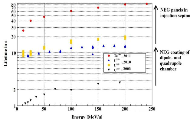
Figure 4: Measured lifetimes of intermediate charge state, heavy ions after NEG coating of the dipole- and quadrupole chambers and after inserting NEG panels in the injection septum.
