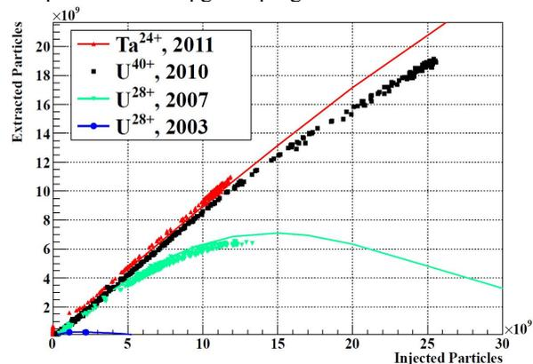
Figure 7: Dependence of the extracted versus the injected number of ions for various stages of the SIS18 upgrade program (measurements and simulations).
