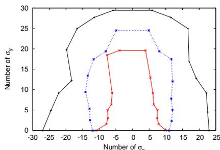
Figure 2: Comparison of the dynamic apertures at the center of the injection region for 10,000 turns in the reference case (black, plus sign), in the case of octupoles in the arc (red, cross sign) and in the case of octupoles in the long straight section (blue, star sign). The rms beam sizes are  $\sigma_x = 1.8$  mm and  $\sigma_y = 0.8$  mm. The amplitude detuning is  $\partial Q_x / \partial \epsilon_x = 425 \text{ m}^{-1}$  and  $\partial Q_y / \partial \epsilon_y = 1155 \text{ m}^{-1}$ .
