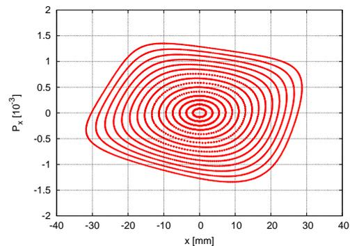
Figure 5: Tracking of a particle with the initial horizontal position  $n\sigma_x$  at the injection point, the other positions are set to zero and  $n$  goes from 1 to 15 with an increment of 1.
