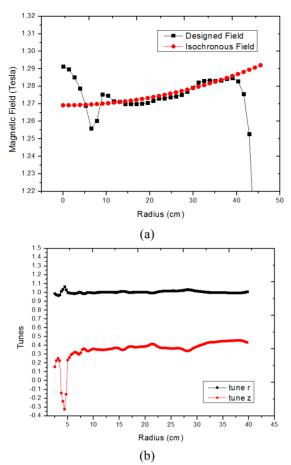
Figure 5: (a)Average magnetic field of magnet with idle isochronous field (b) Radial and axial beam tunes of magnet
