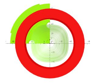
Figure 7: Single turn trajectory of negative hydrogen in electromagnet.
