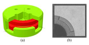
Figure 3: Model body of 13 MeV Cyclotron: (a) Model body before creating mesh. (b) Local meshed model of modeller in OPERA-3D
