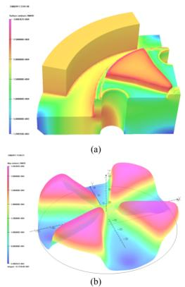
Figure 4: Results of magnetic field calculation with OPERA-3D: (a) Component contour of magnetic field (b) Histogram of magnetic field on mid-plane.
