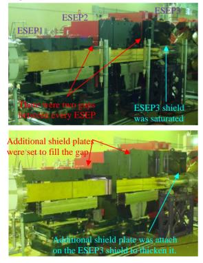
Figure 4: Photo of the ESEPs assembled with the additional shield plates. Upper and lower shows the comparison between before and after shielding.
