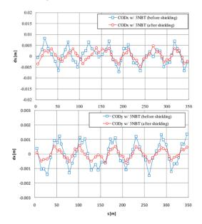
Figure 7: Horizontal and vertical COD measurements at 181MeV storage mode where the 3NBT excited at 3GeV.
