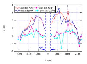
Figure 3: Measured field distribution leaked from the 3NBT-B01 along the s-axis on the top and side of the vacuum chamber, in which the origin indicates the center of the QDL.
