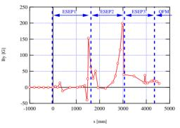
Figure 2: Measured leakage field distribution from the ESEPs along the s-axis on the top of the vacuum chamber, in which the origin of s-axis indicates the upper-stream flange of the ESEP1.
