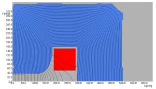
Figure 1: Plan view of half-lamella with flux lines.
