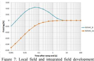
Figure 7: Local field and integrated field developmen after ramping the field to 1.5 T in 500 ms.
