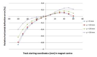
Figure 4: Relative deflection error at 1.5 Tesla.
