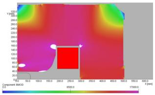
Figure 2: Flux density distribution in lamella at 1.5 T.
