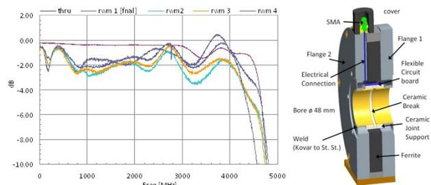
Figure 6: WCM Design and test results of four Monitors.
