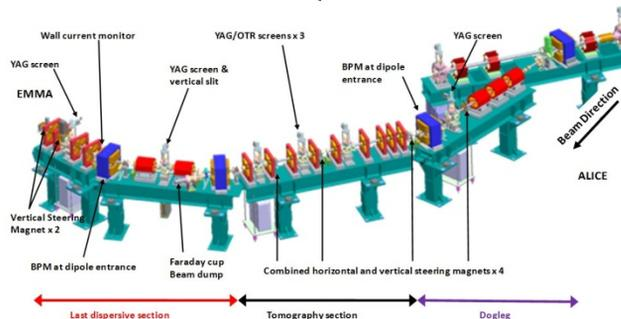
Figure 4: EMMA Injection Line Tomography Section.
