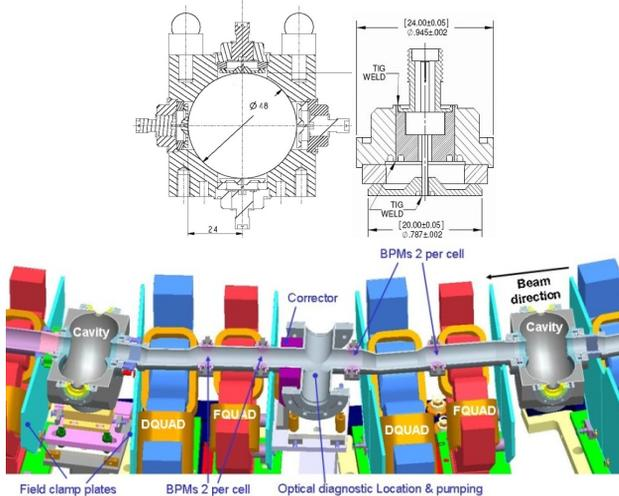
Figure 1: A typical EMMA BPM pickup and Installation.
