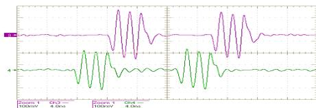
Figure 2: Horizontal and vertical Front-End output doublets.
