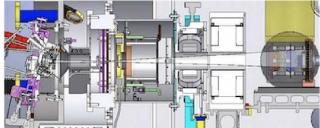
Figure 1: ISHN Ion Source Overview: from left to right: tilted Penning Source, Cs trap section (grey box), post-extraction electrodes (pink), ACCT (orange), DCCT (grey), Quadrupole (light blue), Dipole (white), RPA and Pepperpot (brown).
