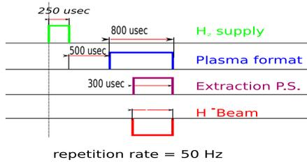
Figure 2: Pulse diagram for beam generation.
