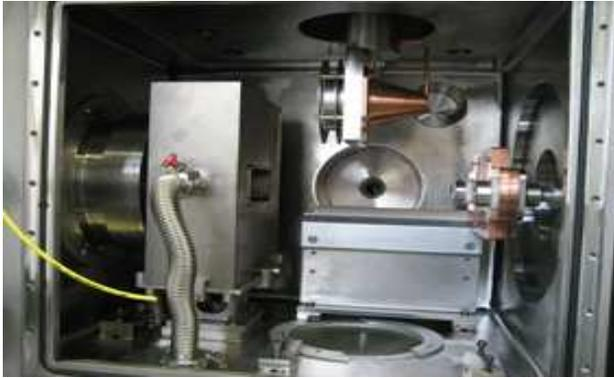
Figure 3: Diagnostic devices: from left to right, ACCT and DCCT (not visible), Quadrupole, Dipole, Faraday Cup, RPA (behind) and Peppercot grid.
