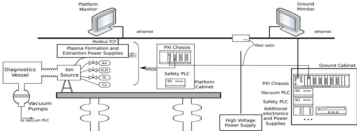
Figure 4: Control system architecture.
