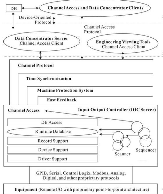
Figure 4: EPICS distributed architecture for the remote control system.
