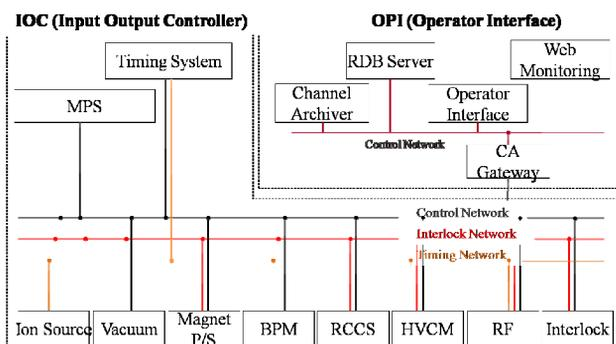
Figure 2: Block diagram of networked control system.
