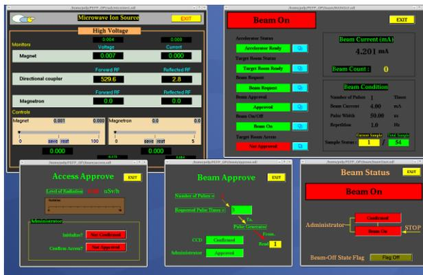
Figure 6: Communication interface for beam operation between users and operators.
