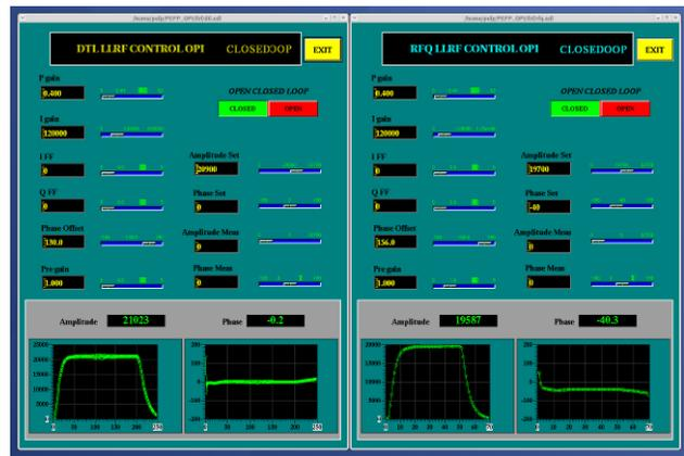
Figure 7: Operator interface for low-level RF feedback control.
