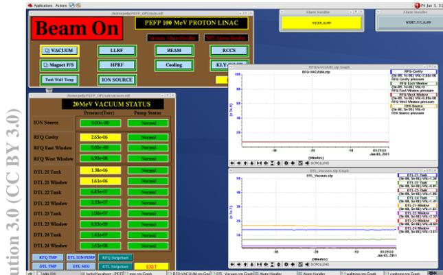
Figure 5: Operator interface using Extensible Display Manager (EDM) for vacuum control and monitoring.
