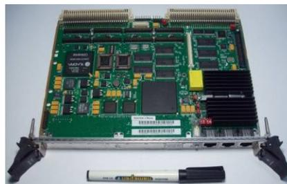
Figure 3: Input Output Controller (IOC) of VME system.
