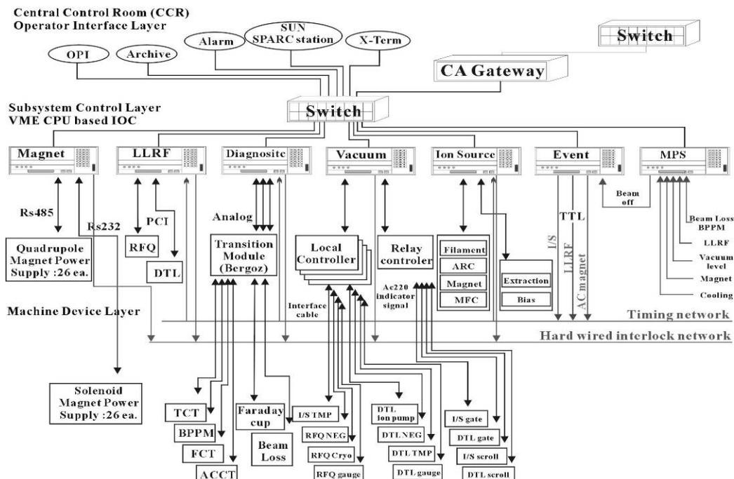
Figure 1: Layout of EPICS-based control system for the PEFP 100-MeV proton accelerator.
