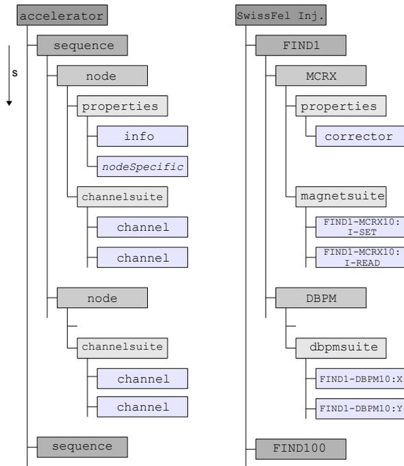
Figure 1: A hierarchical representation of a particle accelerator with associated XML elements (left), accompanied by a partial instance for the SwissFEL Test Injector (right).
