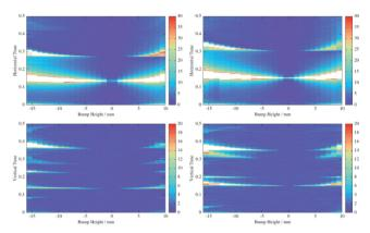
Figure 8: Fourier transforms of beam oscillation of operation point (40.14, 18.35) (left) and (40.15, 18.35) (right). Figures at upper (lower) line represent the horizontal (vertical) oscillation.
