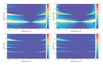
Figure 5: Fourier transform of beam oscillation after kicked by pulse bump magnets.
