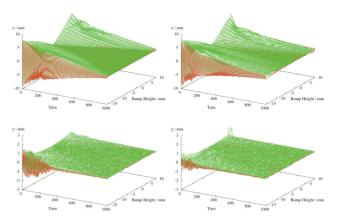
Figure 4: Beam oscillation in time domain after kicked by pulse bump magnets.
