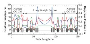
Figure 2: Lattice functions of low emittance optics of the Spring-8 storage ring. The red (blue) line denotes the horizontal (vertical) betatron function and the green one represents the horizontal dispersion function.
