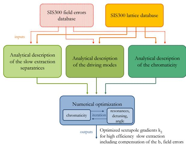
Figure 1: Scheme of the optimization procedure.
