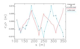
Figure 1: Simulated orbits (points) compared to uncalibrated and calibrated model
