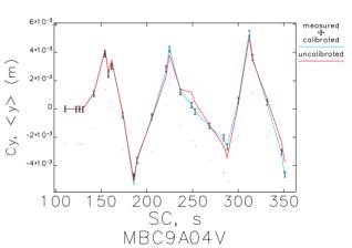
Figure 2: ARC9 measured orbits(points) compared to uncalibrated and calibrated model
