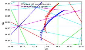
Figure 6: Comparison of measured FM with (red) and without (blue) I09 and I13 optics at  $\xi_x/\xi_y=2/2$ .
