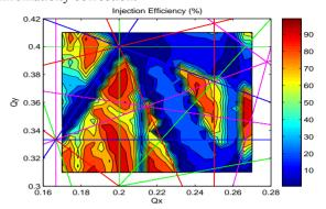
Figure 5: The measured injection efficiency for different tunes with all IDs and collimators closed.
