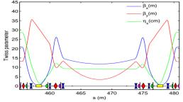
Figure 9: Twiss parameters of I21 optics with  $\beta_y$ =3.4m at the centre of long straight.
