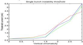
Figure 8: Measured single bunch instability thresholds as a function of chromaticity for I13 (red), I13+I09 (green) and without I09 and I13 (blue) optics.
