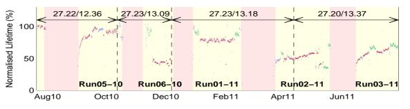
Figure 7: The normalized lifetime during user runs for different optics and fill patterns (900/686 bunches – red/green); Run05-10) unmodified WP= (27.22, 12.36); Run06-10) I13 WP= (27.23, 13.09), Run01-11) I13 WP= (27.23, 13.18), Run-02/-03-11) I09+I13 WP= (27.20, 13.37).
