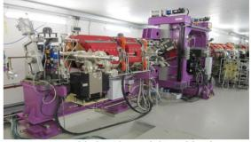
Figure 1: Assembled I13 straight with downstream undulator (coherence) and middle girder with doublet.
