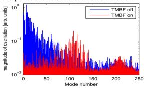
Figure 2: Amplitude of excited modes; blue) without TMBF, red) with TMBF.
