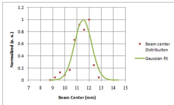
Figure 5: Pulse-to-pulse energy variation: histogram of 100 pulses. The standard deviation of the beam center position is 0.7 mm which equals to a rms pulse-to-pulse energy variation of 0.07%. The peak-to-peak energy variation is  $\pm 0.2\%$ .
