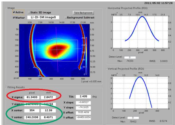
Figure 4: The measured beam size is given in (red circle). Energy spread information can be deduced from the calculated beam size and dispersion relation. The beam center locations (green circle) for each shoot were recorded for stability analysis.
