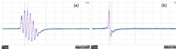
Figure 7: A single bunch beam measured with pickup electrode. (a) The bunch contains six buckets at 0.33 ns distance with similar charge when the SPB is off; (b) The bunch contains one main bucket and only two small neighbour buckets at  $\pm 0.33$  ns (with SPB operating).
