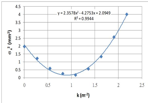
Figure 6: SBM – beam size variation verse Q-1 strength.
