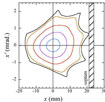
Figure 3: Phase space contour at the injection point of NewSUBARU. The shaded area is the injection septum.
