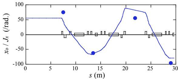
Figure 2: Amplitude dependent orbit shift. The circles are the measured shift and the solid line is the calculated shift using the analytical formula.
