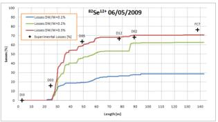
Figure 4:Three theoretical losses curves are plotted with different assumption of energy spread for the input beam. It is visible a good agreement between simulation and measurements with the hypothesis of a tandem energy spread of 0.3%.
