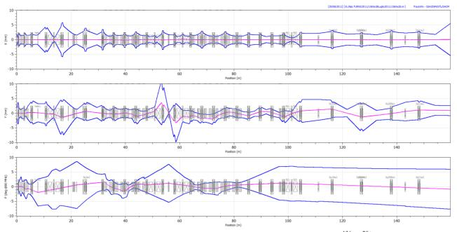
Figure 2: Multiparticles RMS envelopes on X,Y and Phase, in the case of PIAVE-ALPI  $^{136}Xe^{28+}$  in July 2011, from the Exit of SRFQ to the 2° Experimental Hall.
