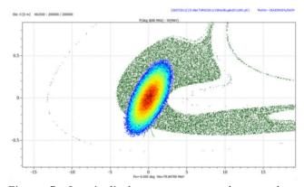
Figure 7: Longitudinal acceptance on the complex PIAVE-ALPI, with the beam injected from the RFQ, for the shit of  $^{136}Xe^{28+}$  of June 2011.
