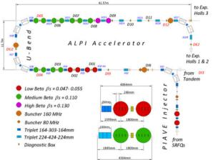
Figure 1: Layout of the PIAVE injector and the ALPI Linac. The three different beta sections of the accelerator are shown in different colours. The change of the lattice length before and after the U-bend is also exposed in the bottom right part of the picture. The names in red for the beam diagnostic box are where the beam current can be measured by a Faraday Cup.
