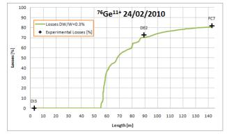
Figure 5:The simulation well predicts the losses also in case of anomalous transport. The bunching was done in the high energy ALPI branch.
