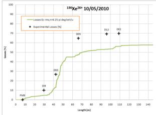
Figure 6:The real injection from PIAVE is affected from problems of misalignment with the ALPI input, and the effects of vertical steering of  $\pm 2$  mm induce a lot of losses after D03.
