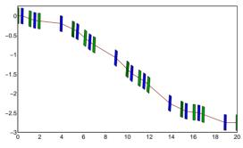
Figure 6: Overall layout of the dogleg variant three. Blue and green colors mark dipole and quadrupole magnets, respectively.
