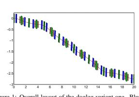
Figure 1: Overall layout of the dogleg variant one. Blue, green and brown colors mark dipole, quadrupole and sextupole magnets, respectively.
