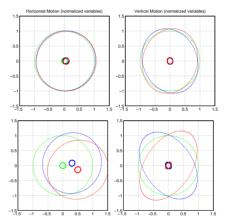
Figure 8: Phase space portraits of monochromatic  $0.1\sigma_{x,y}$ and  $1\sigma_{x,y}$  ellipses (matched at the entrance) after tracking through the dogleg variant three. The relative energy deviations are equal to  $\pm 3\%$  (top) and  $\pm 5\%$  (bottom).
