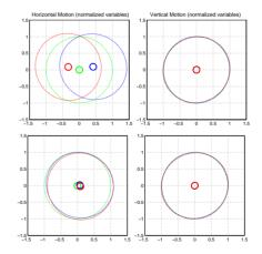
Figure 4: Phase space portraits of monochromatic  $0.1\sigma_{x,y}$ and  $1\sigma_{x,y}$  ellipses (matched at the entrance) after tracking through the dogleg variant one (top) and the dogleg variant two (bottom). The relative energy deviations are equal to  $\pm 3\%$ . Sextupoles are switched off.
