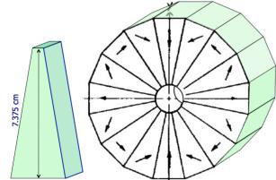
Figure 2. A sketch of the dipole magnet used in constructing the arc lattice for the proton accelerator.
