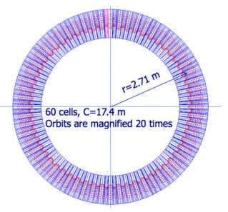
Figure 5. Ring made of 60 cells with permanent magnets. The orbits are magnified 20 times.
