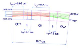
Figure 3. Basic cell of the NS-FFAG made of permanent magnets as presented in Fig. 2.
