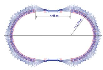
Figure 6. Closed orbits for 31-250 MeV in a racetrack.
