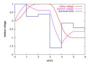
Figure 7. The full cycle with the cavity voltage (red) during the phase jump acceleration. The klystron voltage in shown in pink, while the low level RF drive is shown in blue color.
